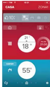
A simple App allows you to manage the water and space heating systems and adapt them to your own needs in a user-friendly way. Switching on, heat level adjustment and time setting are completed in a few easy steps.
